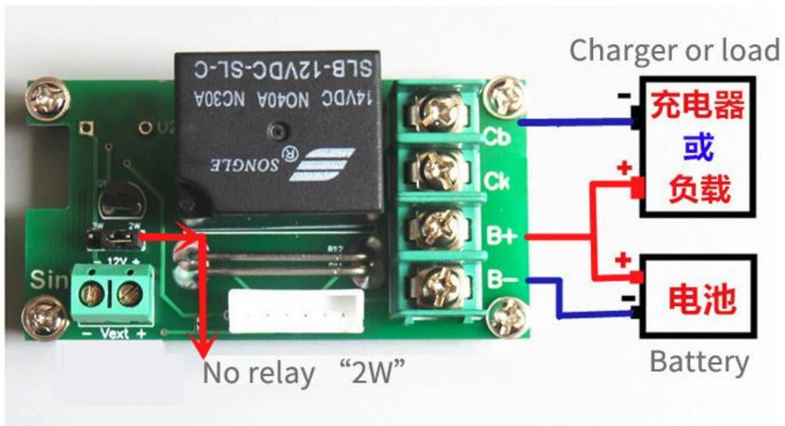
The relay function is not turned on: the positive and negative poles of the power supply and the load (charger) are connected to the common terminal "B+", the negative pole of the battery is connected to the "B-", and the negative pole of the load (charger) is connected to the "Cb". The short-circuit terminal cap can be connected at 2W. Cb is normally closed. If the detection voltage is less than 10V, a 12VDC independent power supply is required to supply power to the meter. Jump the cap to 3W.
